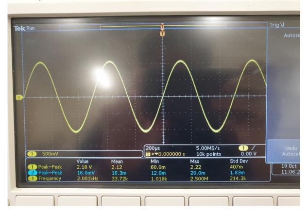
DC biased signal, at the input of the filter. We adjusted the DC bias trimpot to give the waveform a centre-point at around 1.65V (max voltage 3.92V - 2.32Vp-p = 1.6V):
