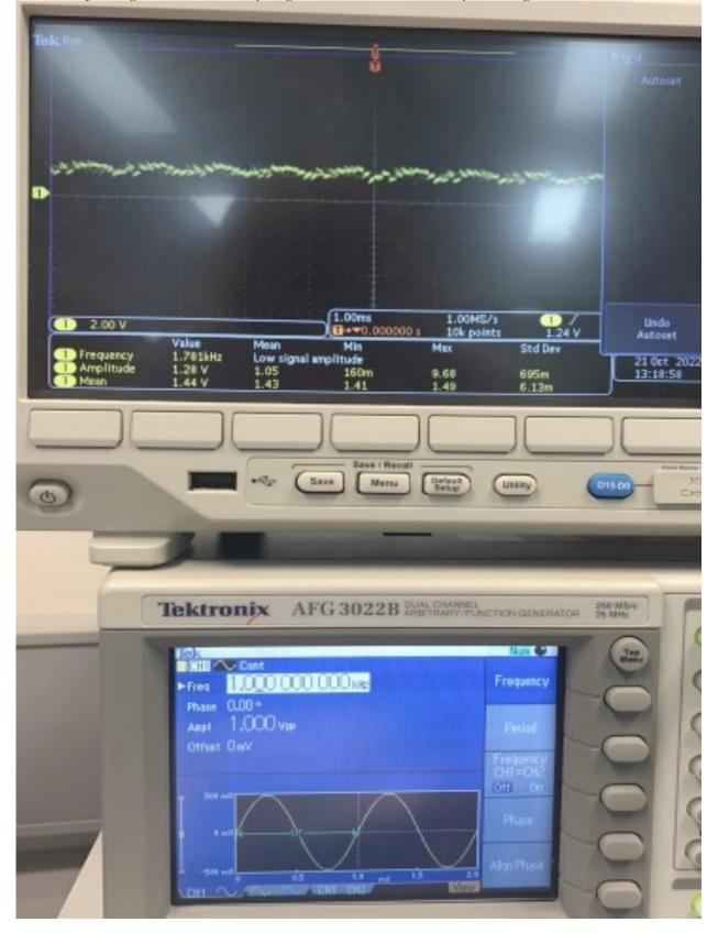
1 kHz input signal, removed by digital FIR filter and only DC signal+noise remains:
